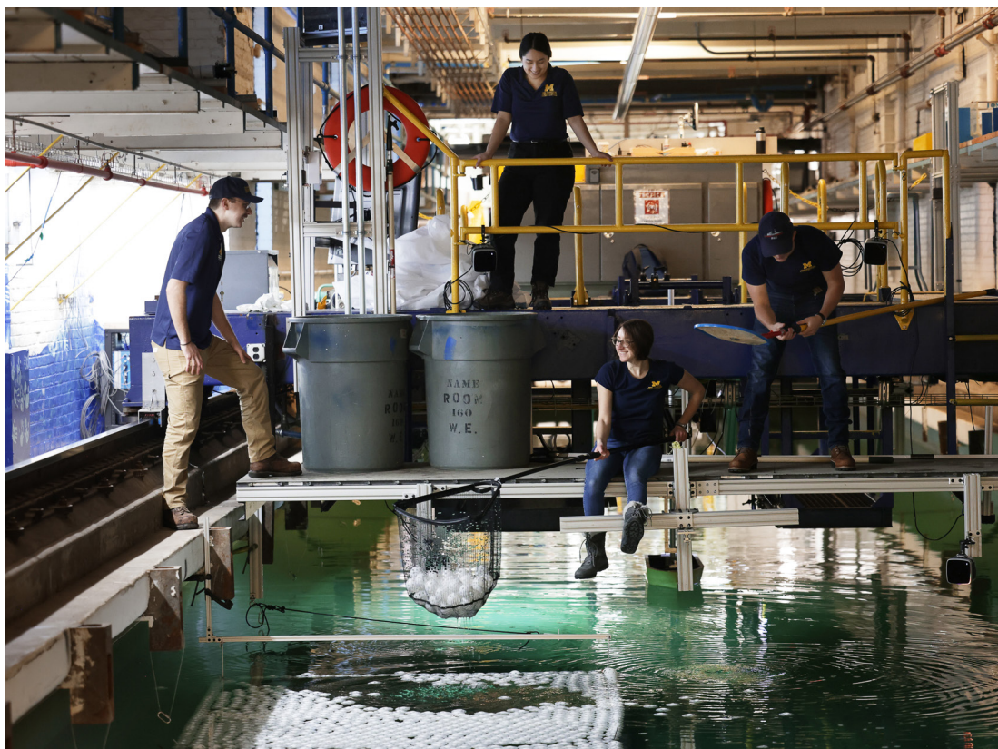
University of Michigan students retrieve “ice” from the university’s tow tank after a day of testing on Feb. 2, 2023. From left to right: Logan Galindo, Victoria Arciniaga, Adina Farca and Jackson Brown. The students researched ship designs for operation in icy conditions as part of a Naval Engineering Education Consortium grant from Naval Surface Warfare Center, Carderock Division. (Courtesy photo by Brenda Ahearn, University of Michigan)
